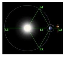
• **Position of the satellite:** In order to get the best science from the sun, continuous viewing of the sun is preferred without any occultation/ eclipses and hence, Aditya- L1 satellite will be placed in the halo orbit around the Lagrangian point 1 (L1) of the sun-earth system.
