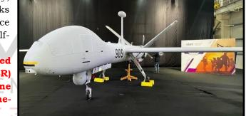
The Drishti-10 Starliner drone, manufactured at Adani Defence's Hyderabad facility, offers a 36-hour endurance and a 450 kg payload capacity. It is the only all-weather military UAV certified with NATO's STANAG 4671 for airworthiness, allowing it to operate in both segregated and unsegregated airspace. The platform supports persistent multi-payload, fully autonomous capabilities and satellite communicationbased operations, crucial for monitoring maritime threats.
